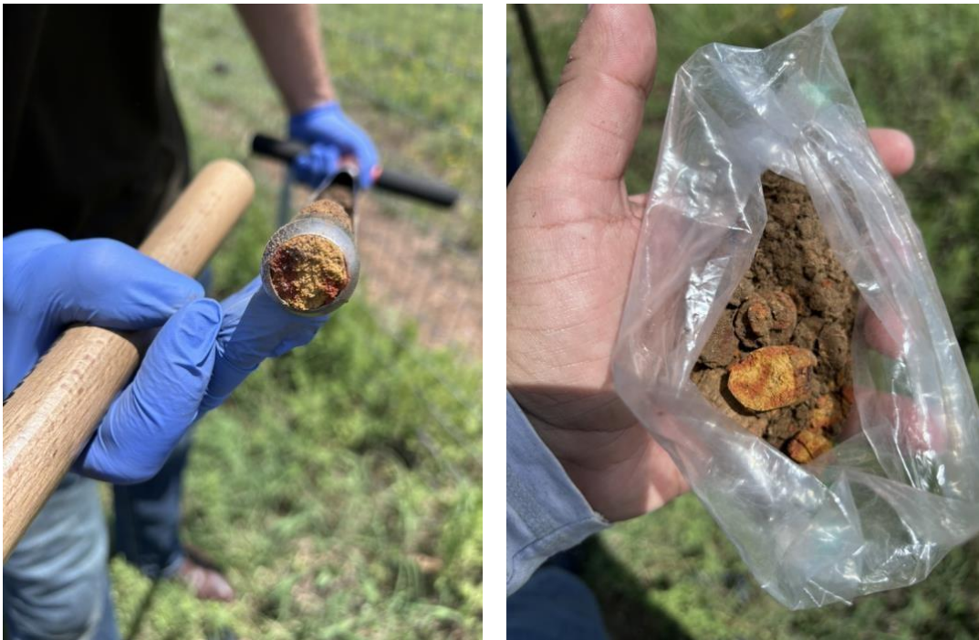
Figure 6. NM05-SD soil cores showing orange iron accumulations and mottled features near the base of the sampling depth. Together with the clay layer and observed site grade, these features support periodic wetness as the leading diagnosis; a field drainage check should confirm it.
